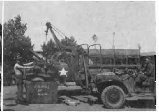
At post war ordnance shop in Ober-Dachstetten, Germany, a two and one-half ton truck gets its engine exchanged. May 1945.
